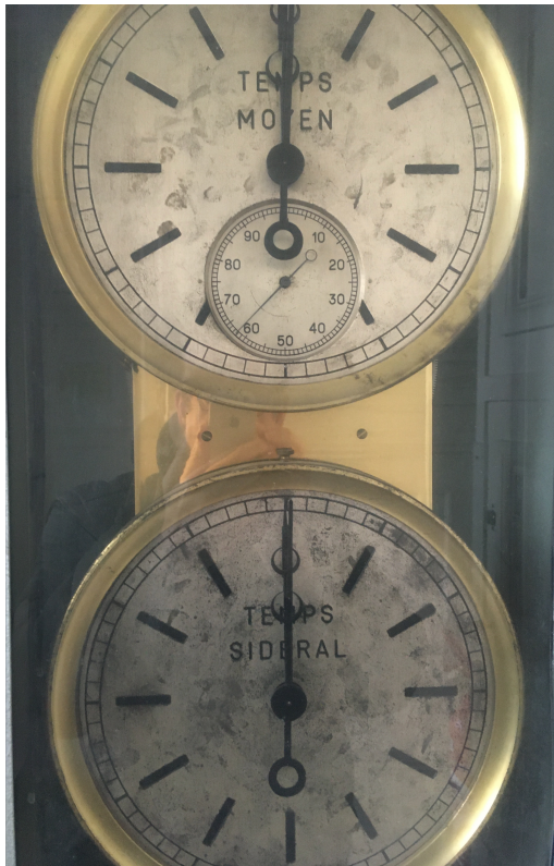
Typical astronomical clock providing Mean solar time & Sidereal time: the Esclançon clock (Paris Observatory, bâtiment Perrault)
